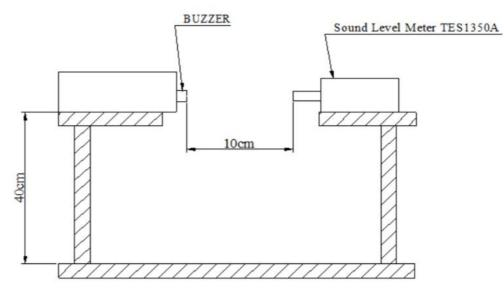
MIC: S.P.L meter TES 1351B or equivalent
