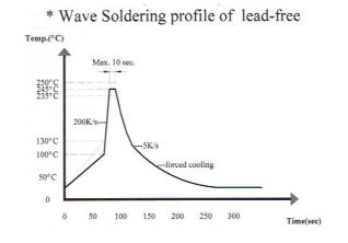
Recommendable wave soldering condition is as follows: Note 1: It is requested that wave soldering should be executed after heat of product goes down to normal temperature. Note 2: Peak wave temperature of 235°C maximum of 10 seconds.
