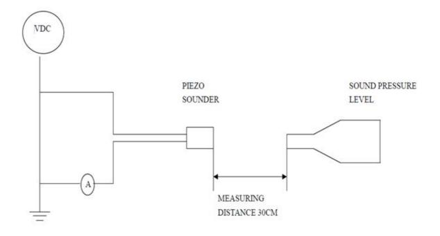
MIC: S.P.L meter TES1351B or equivalent
