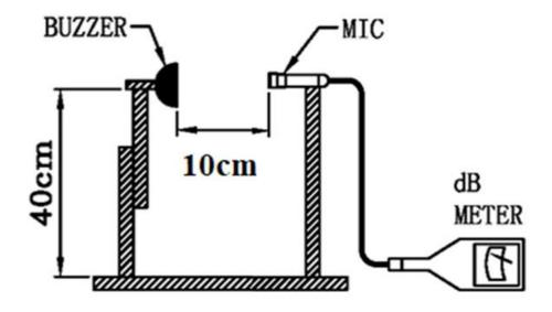
Mic: RION S.P.L meter UC30 or equivalent S.G: Hewlett Packard 33120A Function Generator or equivalent
