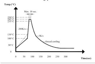
Recommendable wave soldering condition is as follows: Note 1: It is requested that wave soldering should be executed after heat of product goes down to normal temperature. Note 2: Peak wave temperature of 235°C -235°C maximum of 10 seconds.
