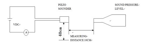
Mic: RION S.P.L meter TES 135 or equivalent S.G: Hewlett Packard 33120A Function Generator or equivalent
