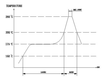
Heat resistant line (Used when heat resistant reliability test is performed)
