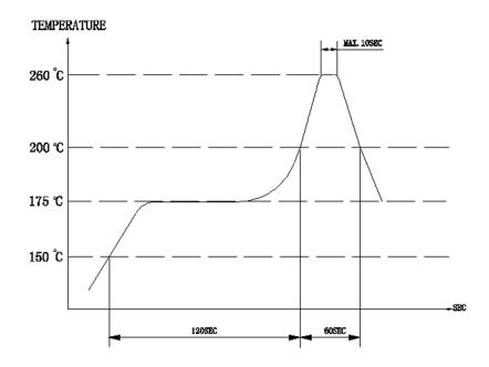
Heat resistant line (Used when heat resistant reliability test is performed)
