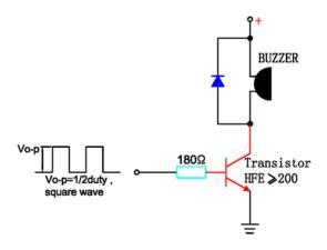
The base current lb should high enough so that it saturates the collector current of the transistor with the CB load.
