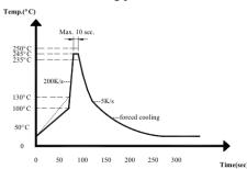
Recommendable wave soldering condition is as follows:
